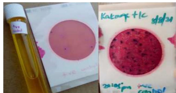
Fig. 4. Positive controls used for the Colilert presence/absence test and the E. coli / Coliform count Petrifilm test.
