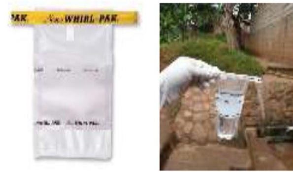
Fig. 2. Collection of water sample from a built water source into a zip-locked 100ml whirl Pak using sterile technique.
