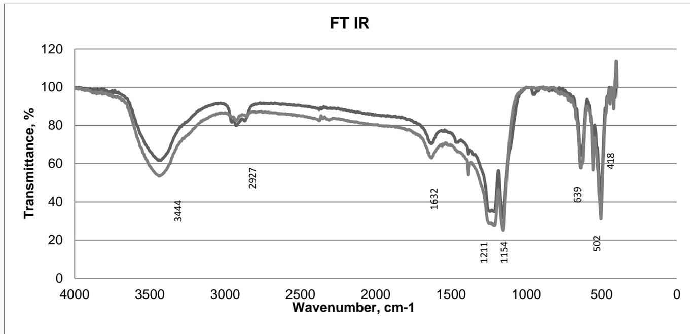
Fig. 2. IR absorption spectra of PTFE: lower – simple 1, upper - sample 2
