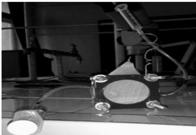
Fig.1. Real reactor of the Microbial Fuel Cell with air cathode
