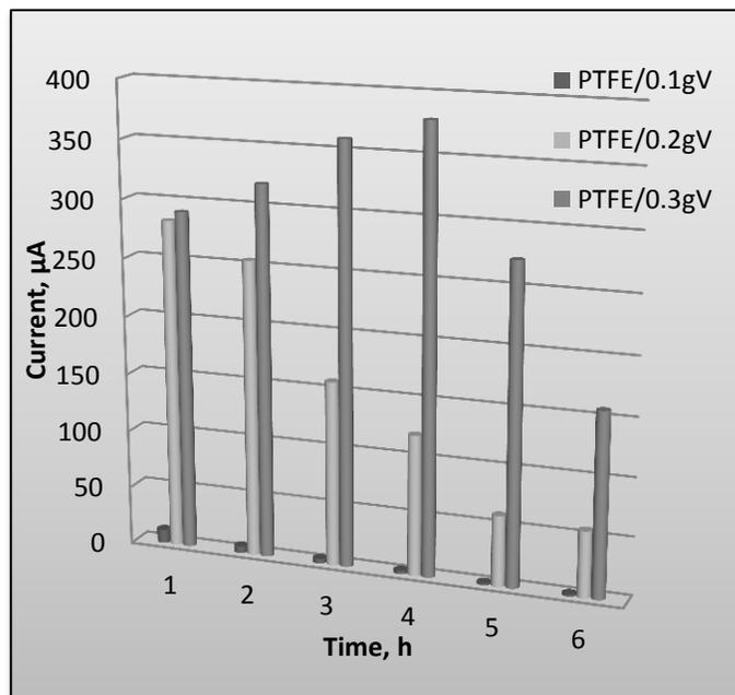
Fig. 4. Current generation in the MFC with three types of cathodes
